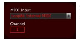
At the left side of the window you will find a panel for choosing a MIDI input port and channel. Through this input, MIDI messages can be received to change the colours of the cubes.
